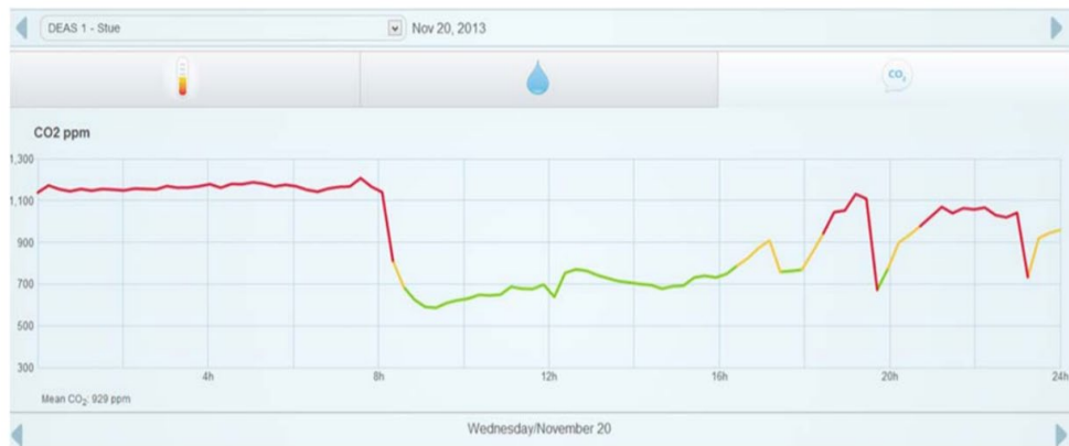
FIGURE 9. CO 2 concentration in an apartment in a 24h period. The concentration is measured every 5 minutes. The colors indicate whether the measurement is within the concentration limits in the green, yellow or red zone respectively [11]. These detailed graphs are only available to the tenants of the individual apartment.
