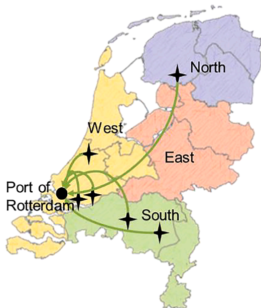
Fig. 4. Simplified representation of distributed configuration of HTL plants and centralized upgrading.
