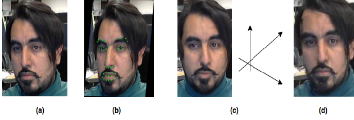
Fig. B.3: Face frontalization process: (a) Query Image, (b) Facial features detection by SDM, (c) Reference face image, (d) Soft symmetry and facial appearance estimation by corresponding symmetric image locations to have frontalized image.
