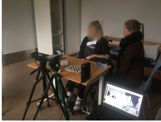
Fig. 2.1: Hardware platform with Axis-RGB, Logitech C920, Axis Q1922-E and Microsoft Kinect V2 for the data collection
