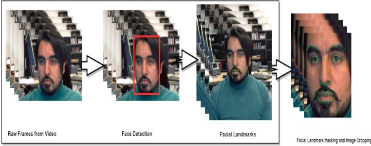
Fig. A.3: Facial landmark identification and tracking in Supervised Descent Method (SDM)
