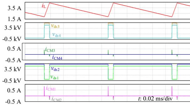
Fig. 4. Simulated waveforms of running BESS
