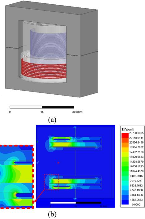
Fig. 9. (a) 3D-CAD model of custom designed transformer and (b) simulated electric field distribution within transformer using ANSYS Maxwell
