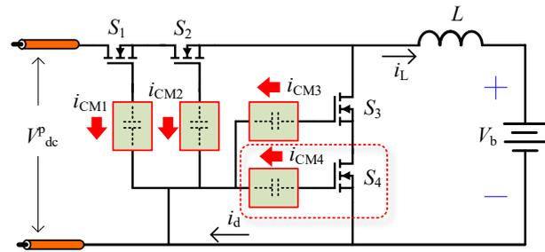
Fig. 2. Bidirectional dc/dc converter in BESS
