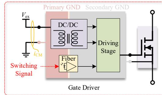
Fig. 3. The gate driver design in a conventional way
