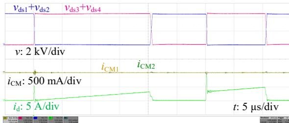
Fig. 15. CM currents of  $S_1$  and  $S_2$  using SCS gate drivers
