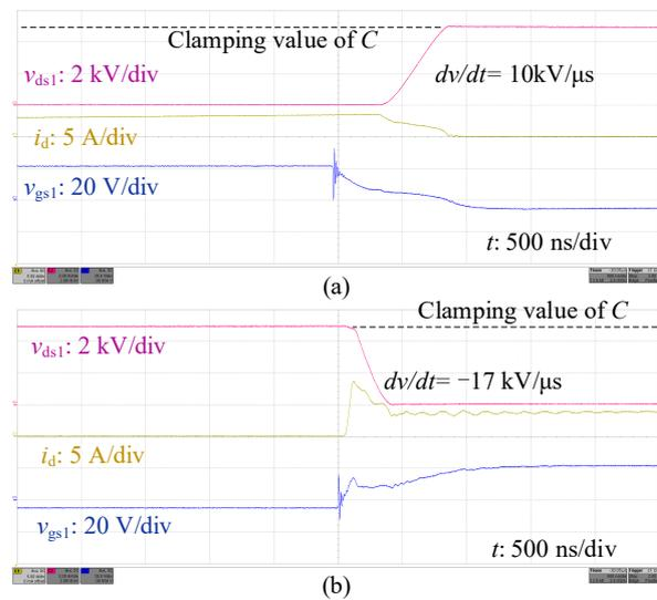
Fig. 13. Measured (a) turn-off (b) turn-on switching waveforms for a 10kV SiC MOSFET using SCS gate driver at 5 kV, 3.5 A
