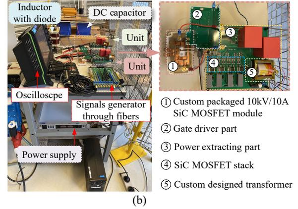
Fig. 10. (a) Schematic and (b) picture of the experimental setup
