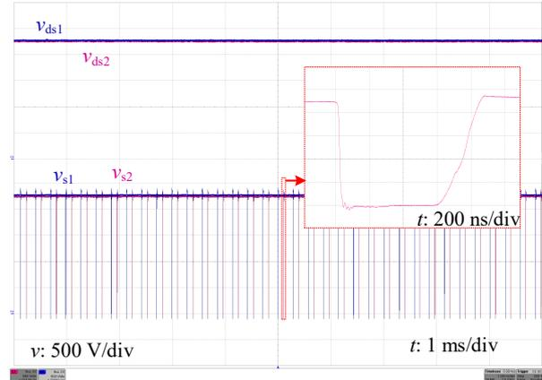
Fig. 16. Measurement showing static voltage balancing of  $S_1$  and  $S_2$  using SCS gate drivers
