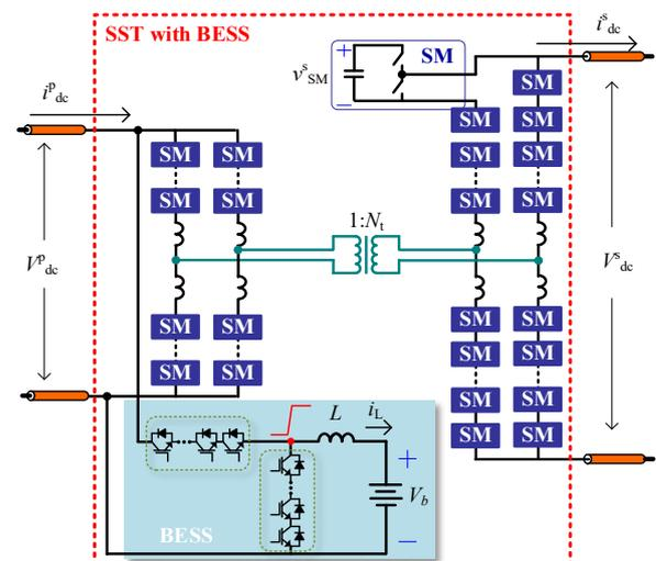
Fig. 1. Configuration of SST with BESS [2]
