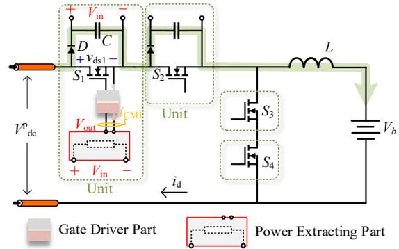
Fig. 5. 10 kV SiC MOSFET based BESS with proposed SCS gate drivers
