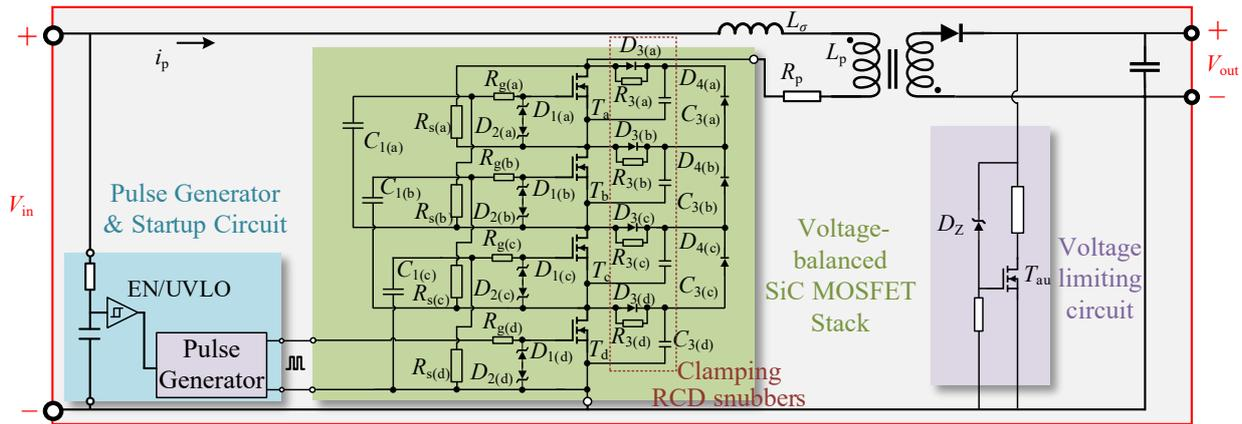
Fig. 6 Power extracting part of the SCS gate driver
