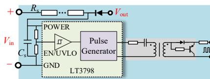
Fig. 8. Pulse generator and its startup circuit
