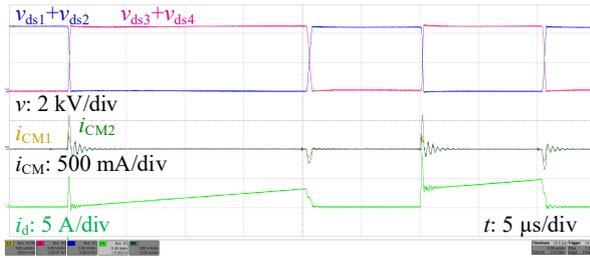
Fig. 14. Measured CM currents for  $S_1$  and  $S_2$  using conventional gate drivers
