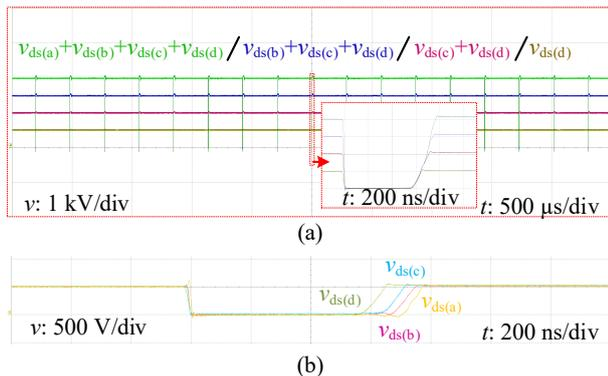
Fig. 12. (a) Zoomed view of Fig. 11 (b) voltage balancing of SiC MOSFET stack
