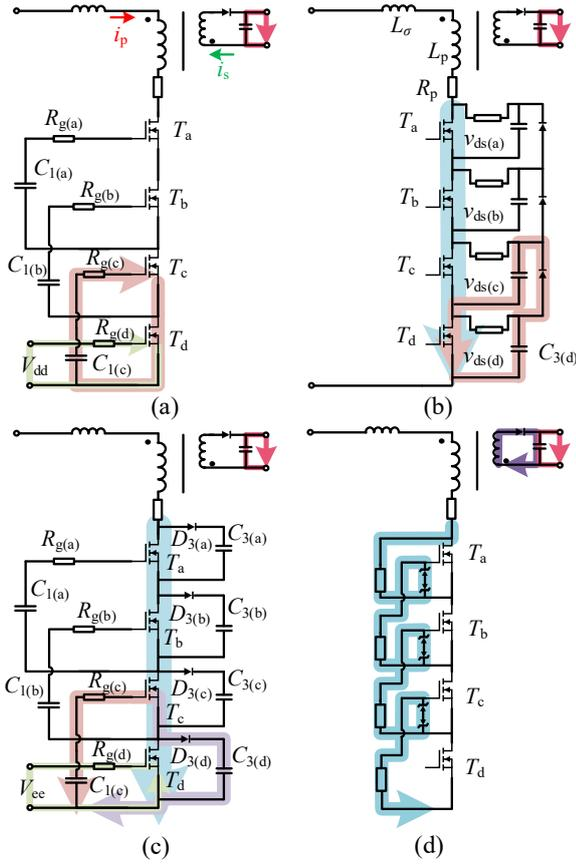
Fig. 7. States of power extracting part: (a) turn-on transient, (b) on state, (c) turn-off transient, (d) off state
