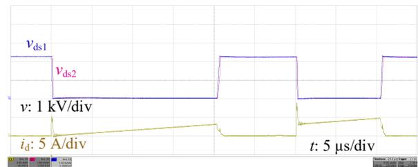
Fig. 17. Dynamic voltage balancing of  $S_1$  and  $S_2$  using SCS gate drivers in a double pulse test
