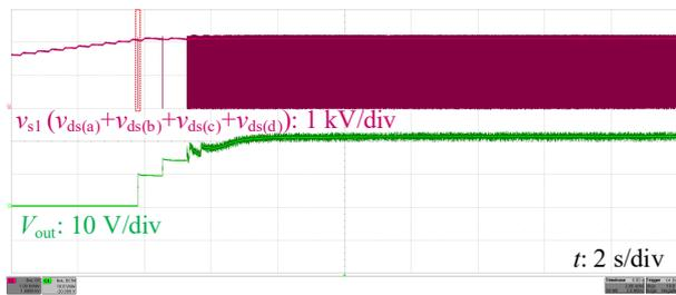
Fig. 11. Startup process using SCS gate driver
