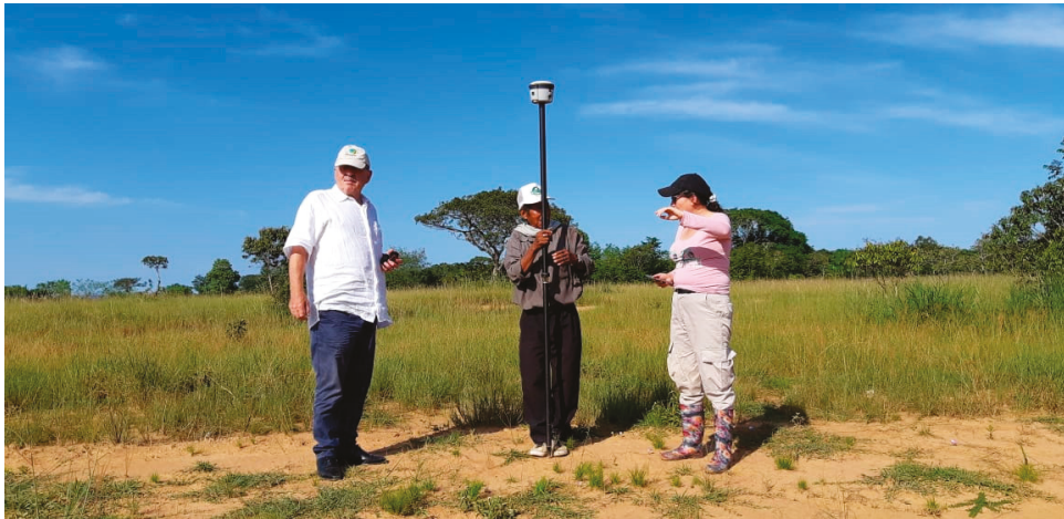
Figure 4. Measuring the boundary of the Santa Teresita del Tuparro reserve with Indigenous leader Horacio Bonilla using a Global Network Satellite Systems (GNSS) antenna. Cumaribo, 2019. Source: Land in Peace Project, Kadaster.
