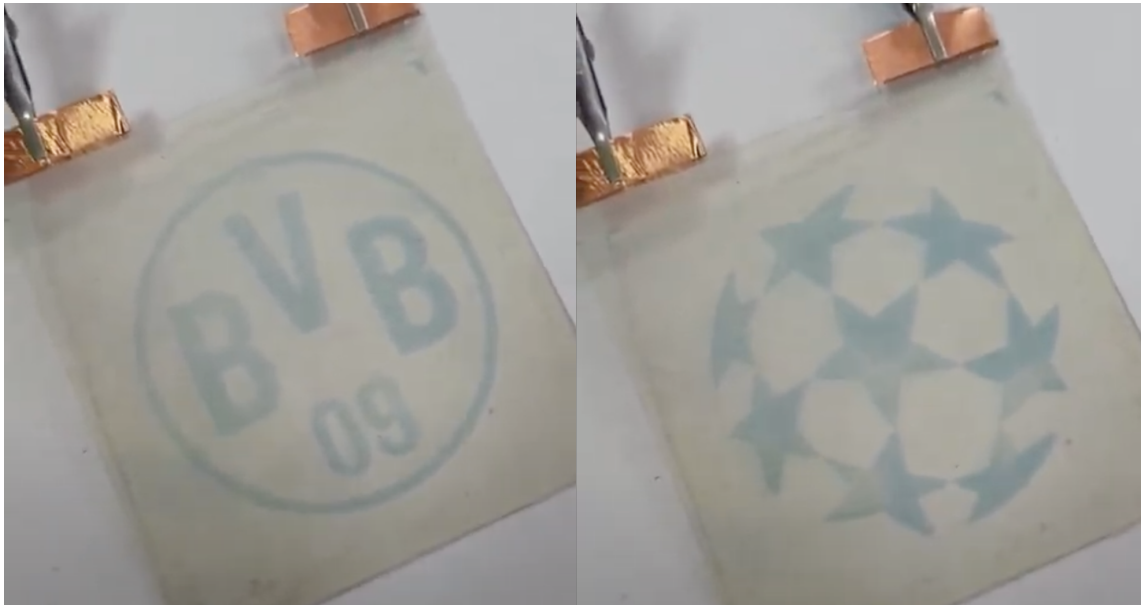
Fig. 2. Example application of EC display with two different states that were created in previous workshops, that allow to switch e.g. a logo, created in [7].
