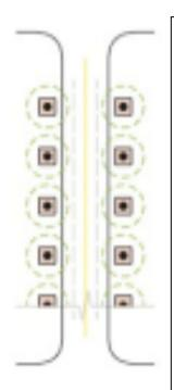
Tree pits placed within the curb, also known as tree trenches, provide multiple benefits, including the collection of surface runoff and the reduction of the urban heat island effect. Since tree roots are not used to growing within compact urban environments, permeable pavement or amended soils can be used to enhance their growth.
