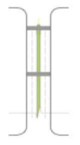
A depressed median, designed to collect and store stormwater, is engineered to direct the flow of water to basins within the median. Medians can double as pedestrian space if integrated with crossings.
