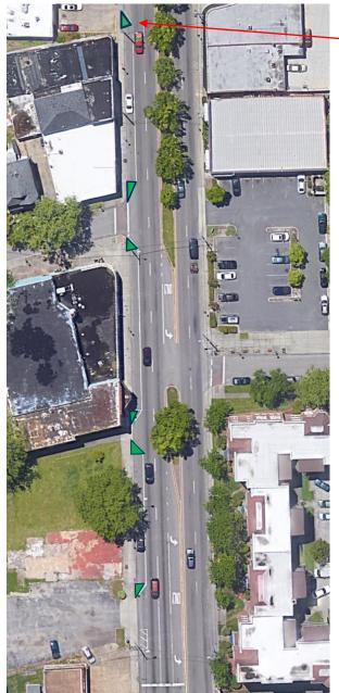
Curb extension planters placed continuously at end of street parking strips
