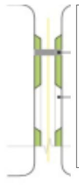
A swale extended from the curb can catch stormwater and serve as a traffic calming device. Swales can also be built into crossings at midblock locations. The curb extensions can be broken up to include parking spaces or placed on one side of the street only.
