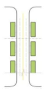
Vegetative planters located within the curb can be independent (flow through) or connected to link up with a larger drainage or retention system. The walls can be made of pavement or more natural materials like stones. Building within the curb, sometimes adding a small strip of pavement between the sidewalk and planter, retains on street parking. Planters can float independently like rain gardens or can be linked together by a small grade and gravity.
