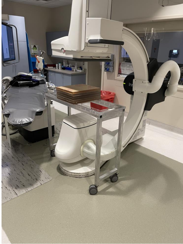
Figure 1: Shows the setup of the study with 6 inches of PMMA on top of the cutout in the correction location over the x-ray tube with the patient table removed.
