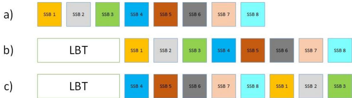
Figure 15. SSB transmission methods in NR-U. a) correspond to intended transmission b) correspond to shifted transmission and c) correspond to wrapped transmission.
