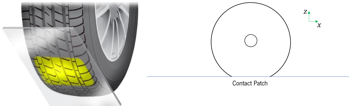
Figure 3.1 - Graphical representation of the tire contact patch. Adapted from (Contact Patch, s.d.).
