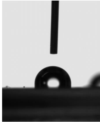
Figure 74 - Water droplet placed on top of a non-microstructured PC surface with the coating application (WCA = 109,2^\circ ).
