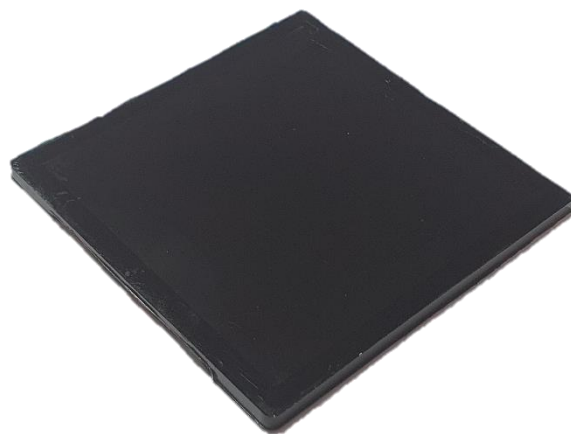
Figure 45 - Representative non-microstructured PC sample used in the replication process for obtaining microstructured parts (50 x 50 x 2 mm).
