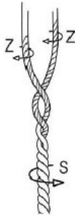
Figure 12 - Twist directions in a greige cord (11).
