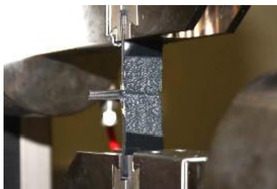
Figure 37 - Tensile machine separating the rubber specimen.
