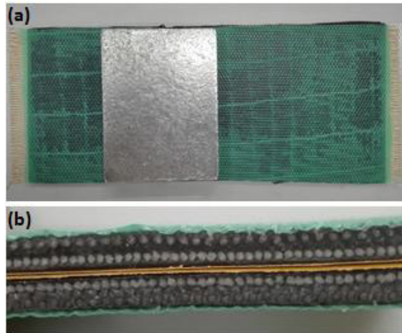
Figure 36 - (a) Peel test specimen after pressurized; (b) lateral view and materials identification.
