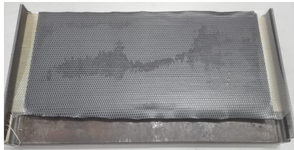
Figure 35 - Peel test specimen preparation.
