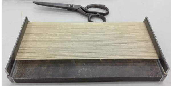
Figure 34 - Textile comb with nylon 940x2 dipped cord.
