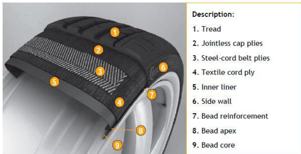
Figure 3 - Typical radial tire cross section (adapted from (5)).
