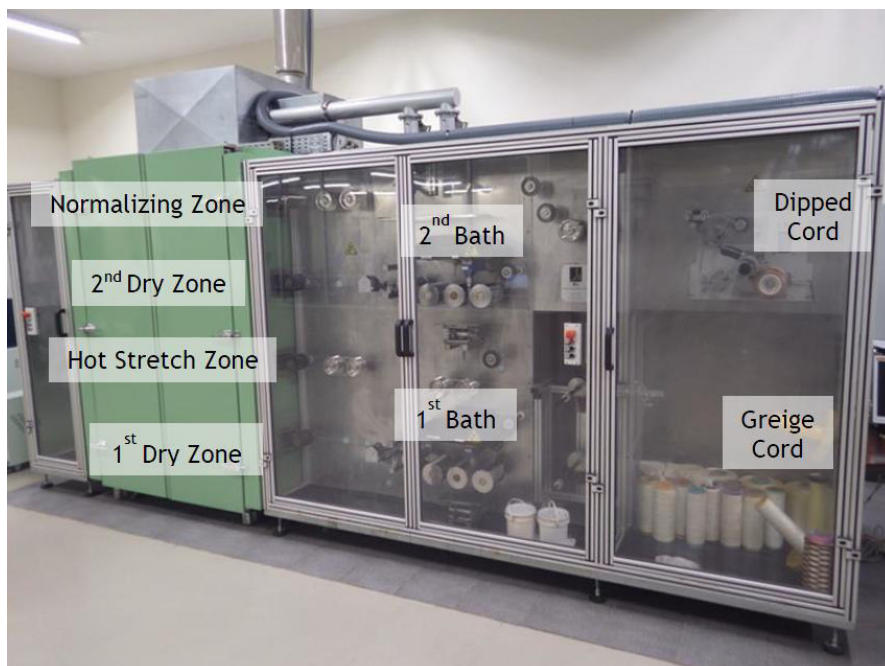
Figure 32 - Laboratory Dipping Unit (LDU) at ITA (48).
