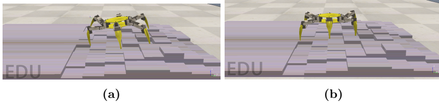
Figure 6. Hexapod posture during the simulation: (a) non-adaptive control and (b) with posture control.
