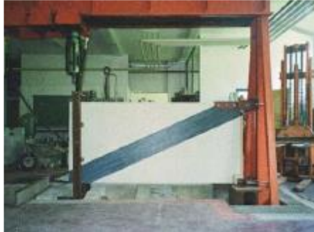
Fig. 9 Walls strengthened with CFRP [18].
