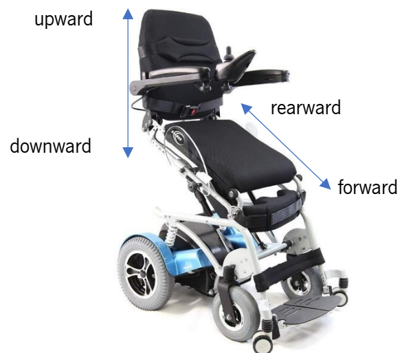
Figure 100 – Directional references signalled in a stand-up wheelchair. (adapted from [32]).
