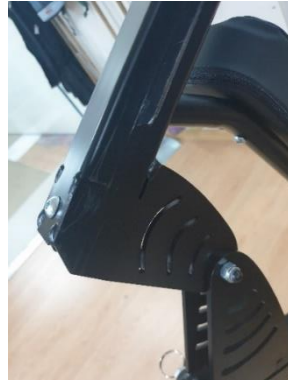
Figure 84 – Structure scratches due to backrest's lack of clearance.
