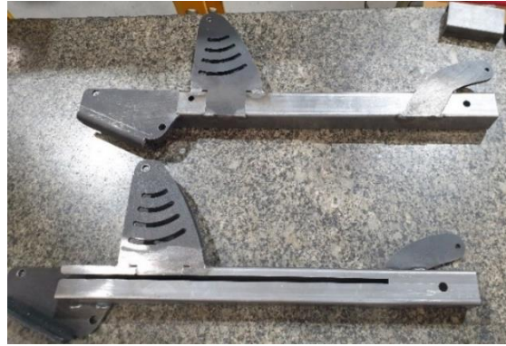
Figure 73 – Example of components after cleaning and deburring the weldment.
