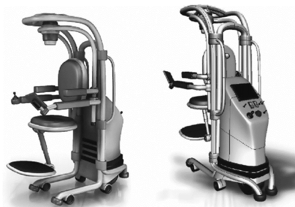
Figure 9 - 3D model of robotic Patient Transfer and Rehabilitation Device (adapted from [42]).
