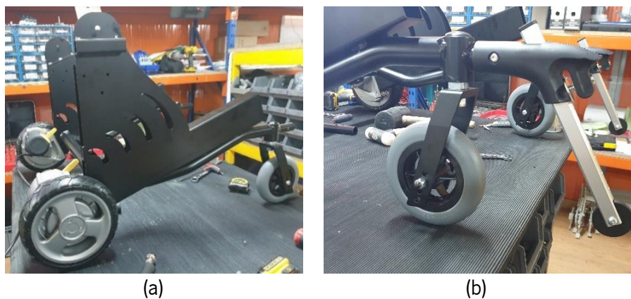
Figure 75 – Chassis assembly: (a) front drive wheels and rear wheels, (b) anti-tippers placement.
