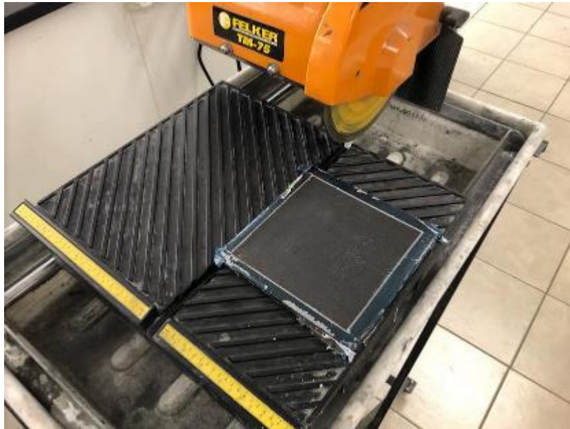
Figure 27: Untrimmed Laminate on Cutting Table
