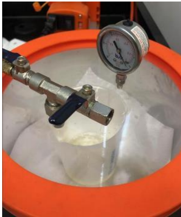
Figure 23: Resin Degassing in Vacuum Chamber
