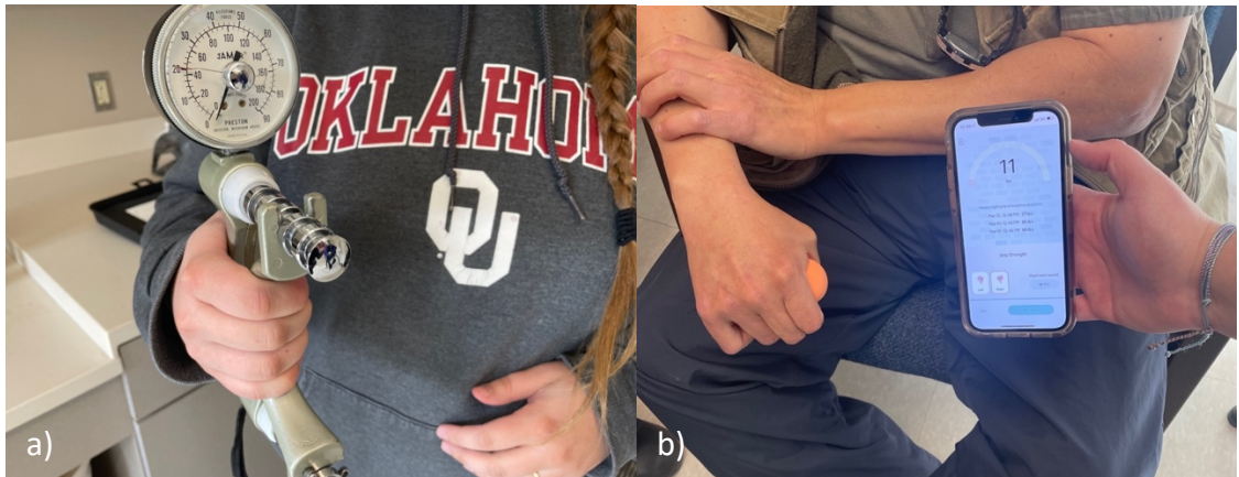
Figure 8. Grip strength measurement using a) the dynamometer, and b) the Squegg device.
