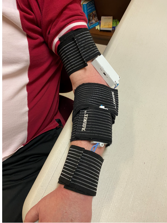
Figure 4. FoVi device secured to participant's arm using Velcro straps.
