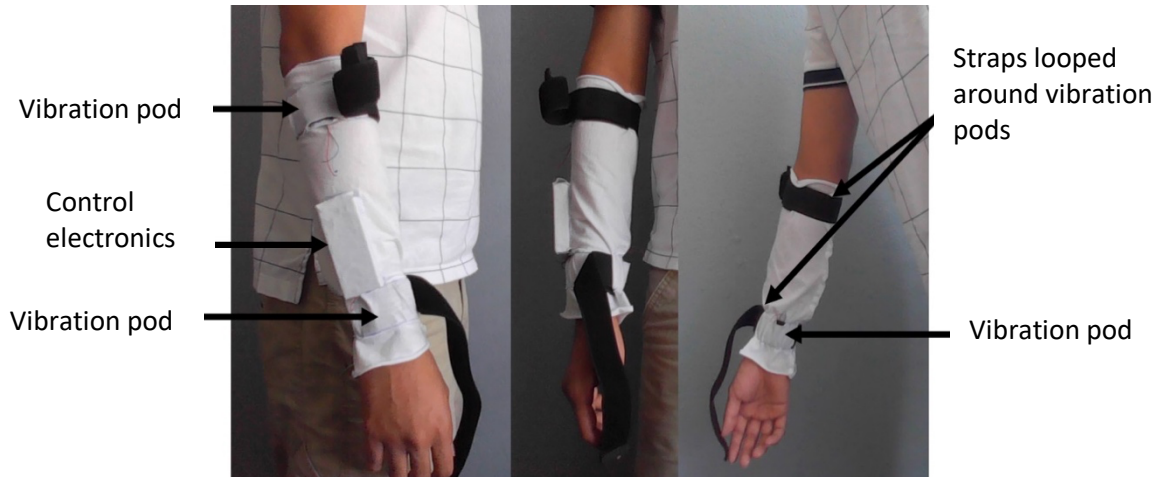
Figure 2. Sleeve design with vibration pods and control electronics box in pockets. Velcro straps are looped around the vibration pods and can be tightened with the other hand. (Wang et al. , 2022)
