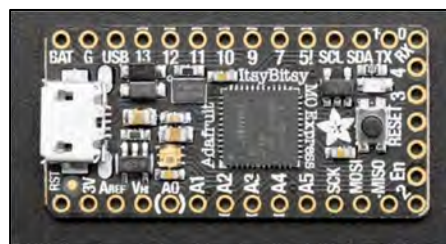
Figure 2.3.2 - Adafruit ItsyBitsy M0 Express development board for the Cortex M0
