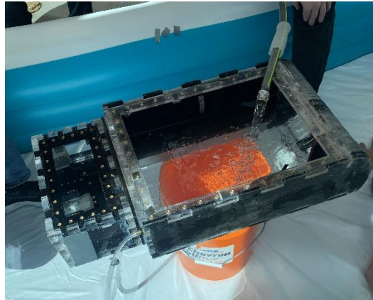
Figure 44. Initial waterproof test of the body
