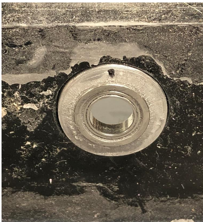
A 12. Marine Grease used for lubrication of locomotion system
