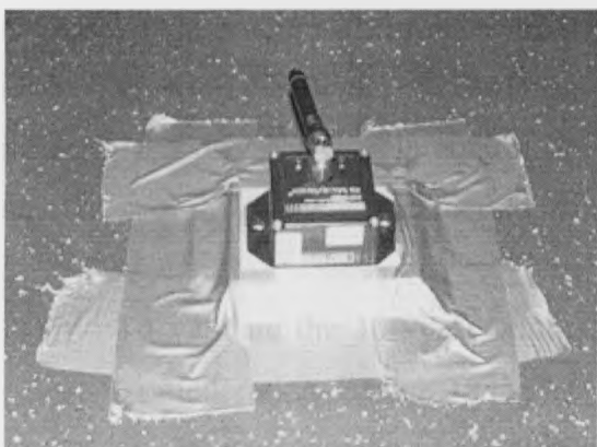
c) Triaxial Accelerometer Bus Floor
