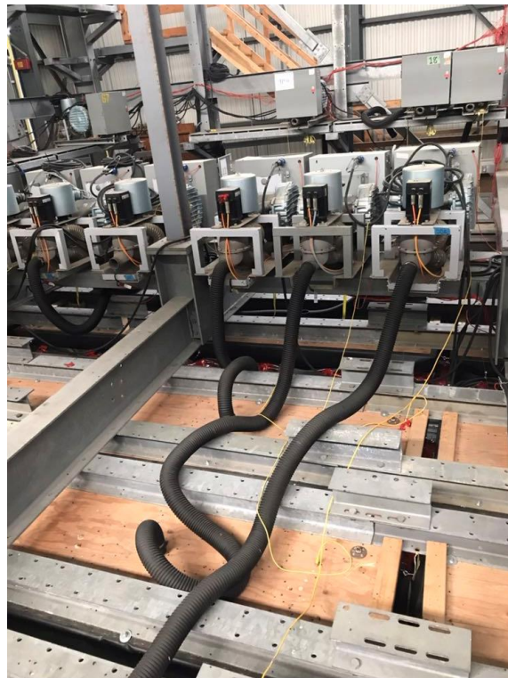
Figure 3.6: Setting up the Pressure Loading Actuators (PLA).
