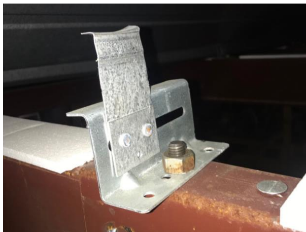
Figure 4.10: Slippage between seam and clip (clip 122).
