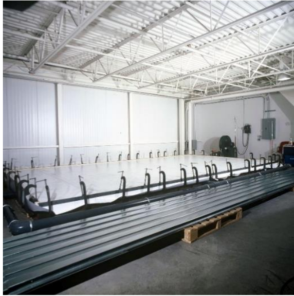
Figure 1.8: Test setup of FM 4474 (Sika, 2015).
