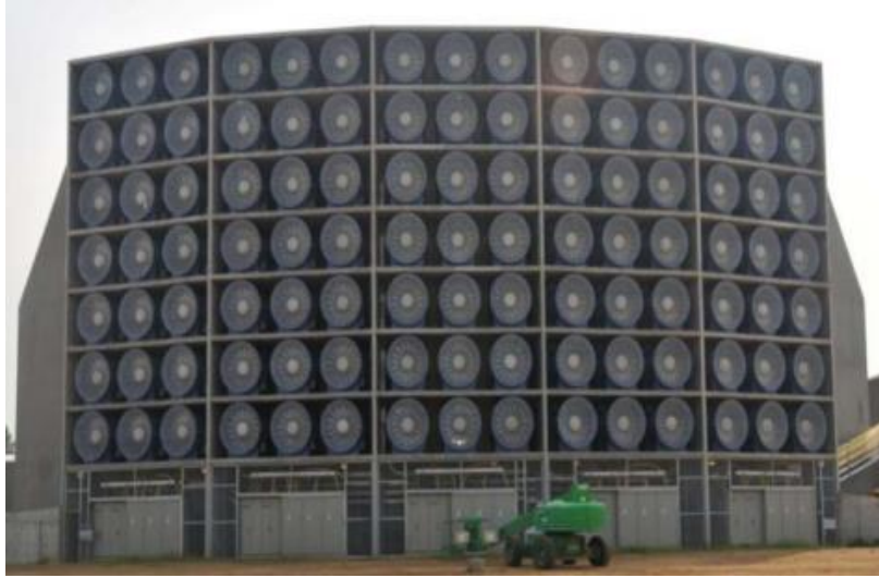
Figure 2.18: Photograph of the full-scale wind tunnel at IBHS (Morrison et al., 2013).
