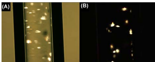
Figure 8.2: Optical micrographs of unpassivated nanowire suspension inside a 0.5mm i.d. glass capillary tube imaged under (A) partial and (B) full cross-polarization.
