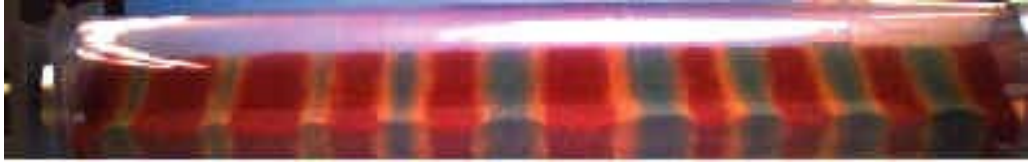
Figure 2.1: An initially uniform mixture of glass beads of three sizes [0.5 mm (blue), 1 mm (gold), 2 mm (red)] segregated into bands. The particles were rotated about an axis perpendicular to gravity at 30 rpm for several hours [88].
