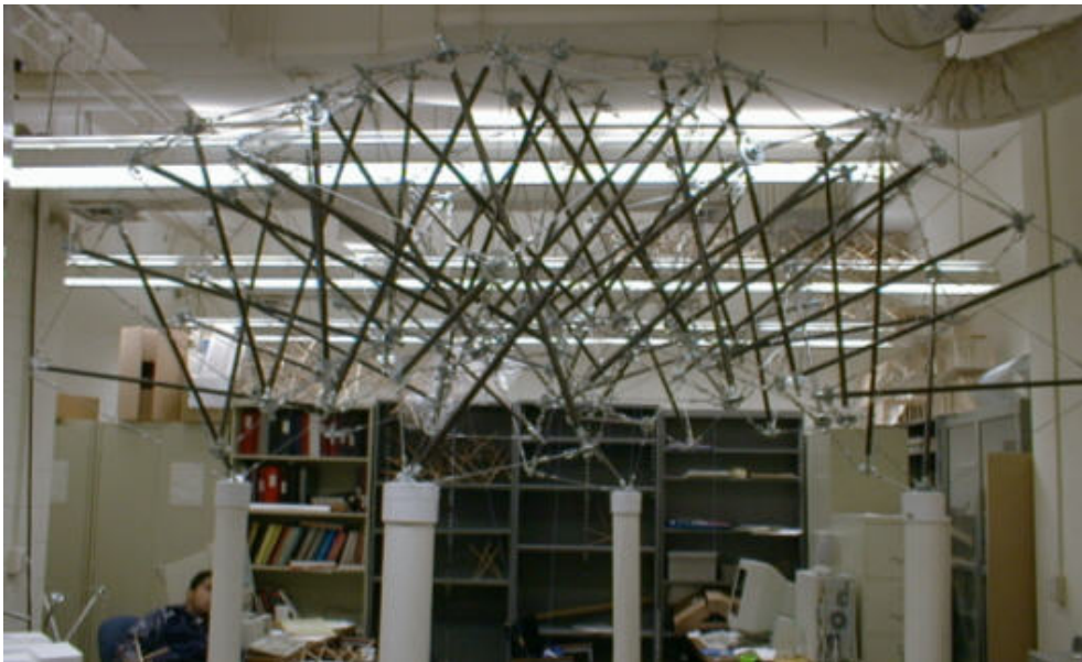
Figure 1-1: Full scale experimental model composed of 16 units (designed and built by K. A. Liapi)
