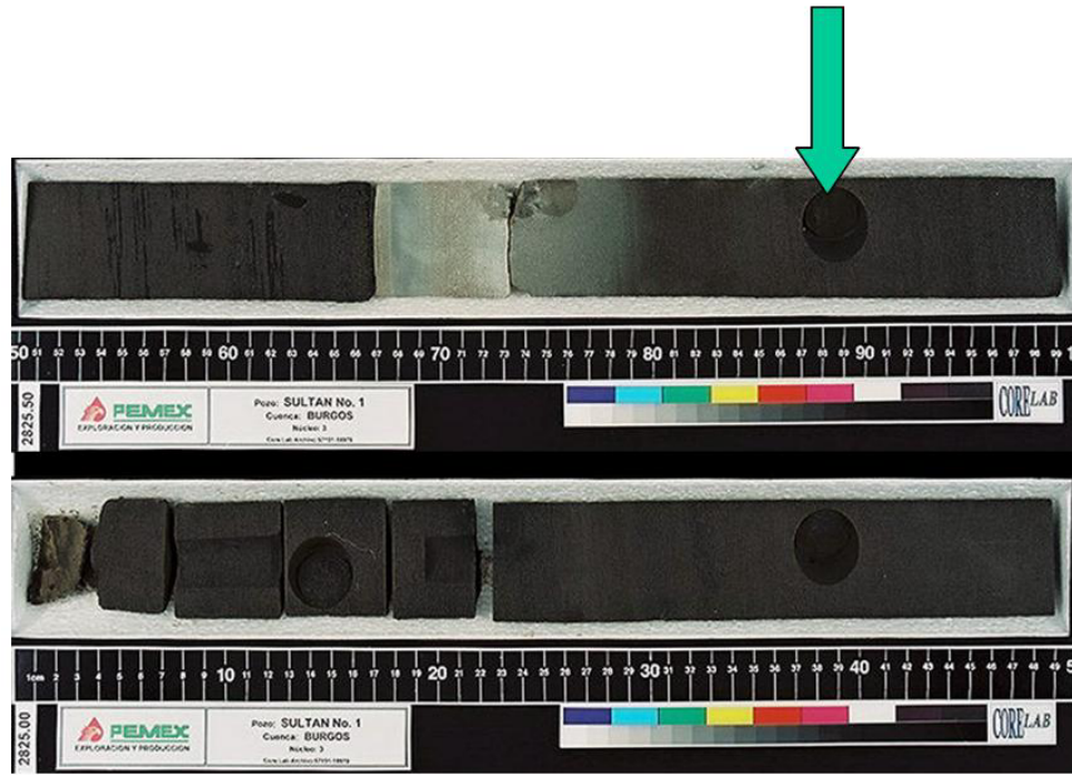
Figure 3.5 Core petrophysical analyses at reservoir interval in S-1 well. Laboratory measurements include bulk, Young, and shear moduli.
