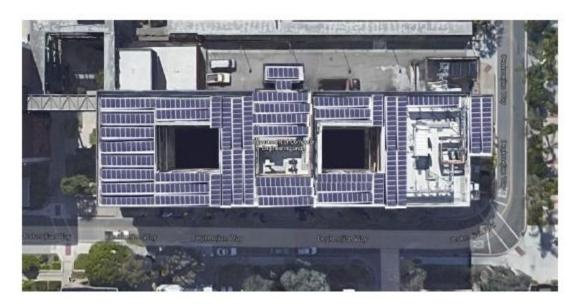
FIGURE 27: Proposed PV system on the roof of the ECS building.
