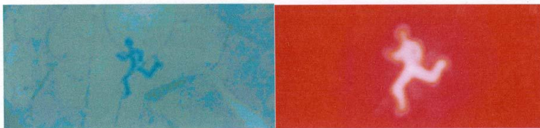
Figure 1.33 Left: VIS-absorption spectrum of the “runner” (DHI ( 1.5.1 )) in PMMA after writing with a 355 nm laser beam. Right: Fluorescence spectrum from the “runner”, excitation at 532 nm. 19
