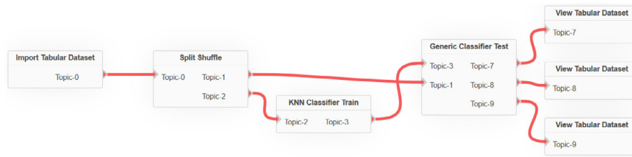
Fig. 5. Snapshot of the workflow of the classification of the Iris dataset in the graphical tool. The first step is when the dataset is loaded. Then, in the second step, the data are split into train and test data. After that, as the third step, train data are used to train a machine learning model and, in the fourth step, both test data and the model are used to test the classifier's prediction. Finally, some useful metrics derived from the model are highlighted.
