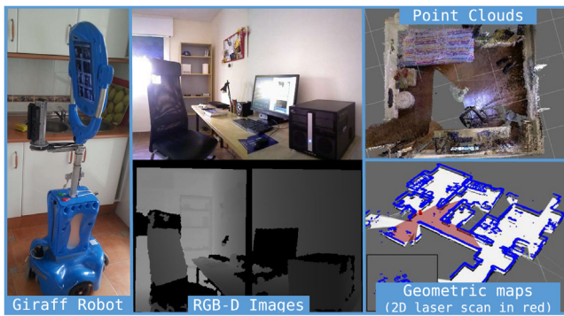
Fig. 7. Mobile robot used to collect the Robot@Home dataset along with some samples of the data it provides.
