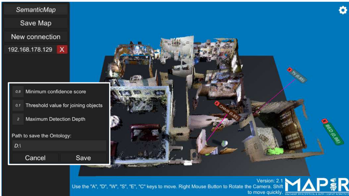
Fig. 4. Graphical User Interface designed to support human–robot interaction including buttons, text fields, and a visualization of the virtual environment with different mechanisms for its modification. Down left, a screenshot of the floating window permitting an advanced configuration of the system.
