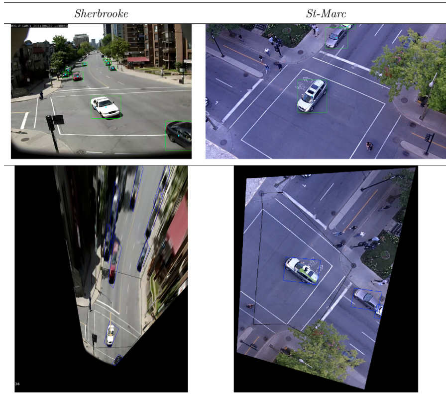
Fig. 7. Qualitative results. First row shows original images (frame 34 from Sherbrooke and frame 894 from St-Marc ) with vehicles detected by fasterv2 . The second row shows the same images after the perspective is corrected by means of the homography. The images shows the coordinates used to create homography (polygon marked as black lines), and the tracked vehicles shows their last trajectory.
