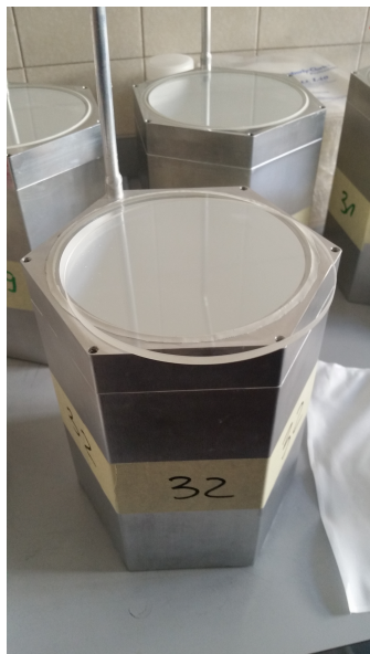
FIGURE 7.4: Checking the crystals of the NEDA detectors.
