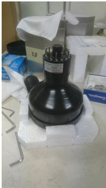
FIGURE 7.11: Photo Multiplier (PM) tube to be coupled to the detector active volume to get the complete NEDA detector assembly.
