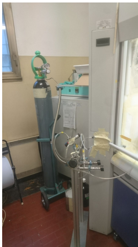
FIGURE 7.6: The pressure system of the NEDA detectors bubbling process.
