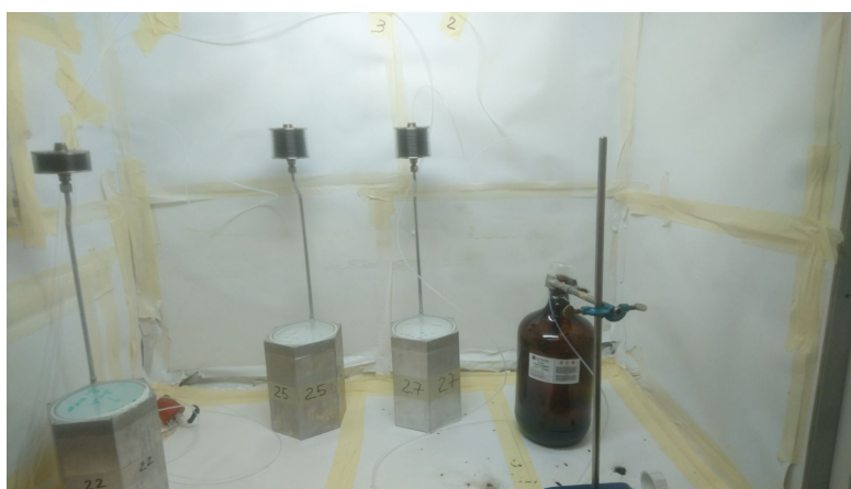
FIGURE 7.5: Bubbling process using NEDA detectors and liquid scintillator bottle.
