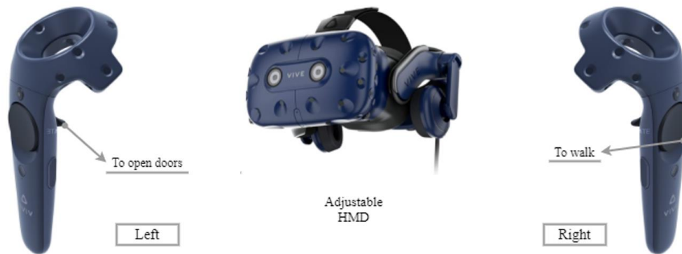
Figure 4 - HTC Components and Associated Controls
