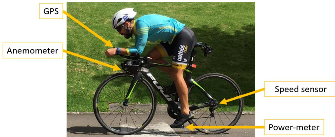
Figure 3.3. Setup for the implementation of the protocol to measure aerodynamic drag.
