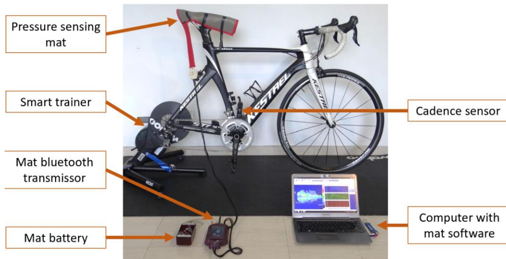
Figure 5.1. Setup for the measurement of pressure in contact areas.
