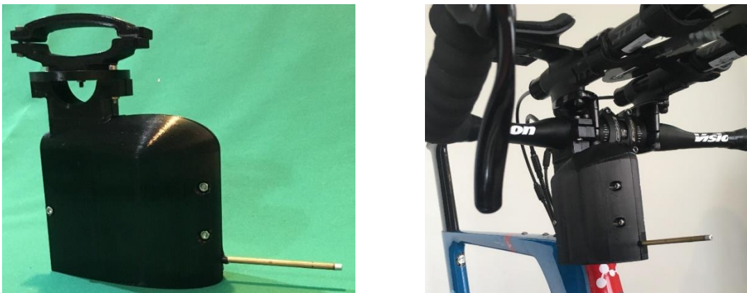
Figure 3.2. Anemometer developed for the estimation of drag area in cycling.
