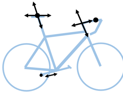
Figure 2.4. Variation of posture due to the location of contact points defined by the bicycle geometry.
