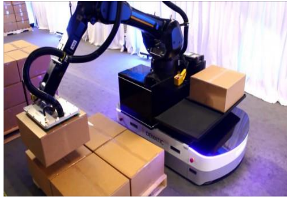
Figure 2. An AGV unloading boxes. Source: Interact Analysis “Mobile robots 2018”
