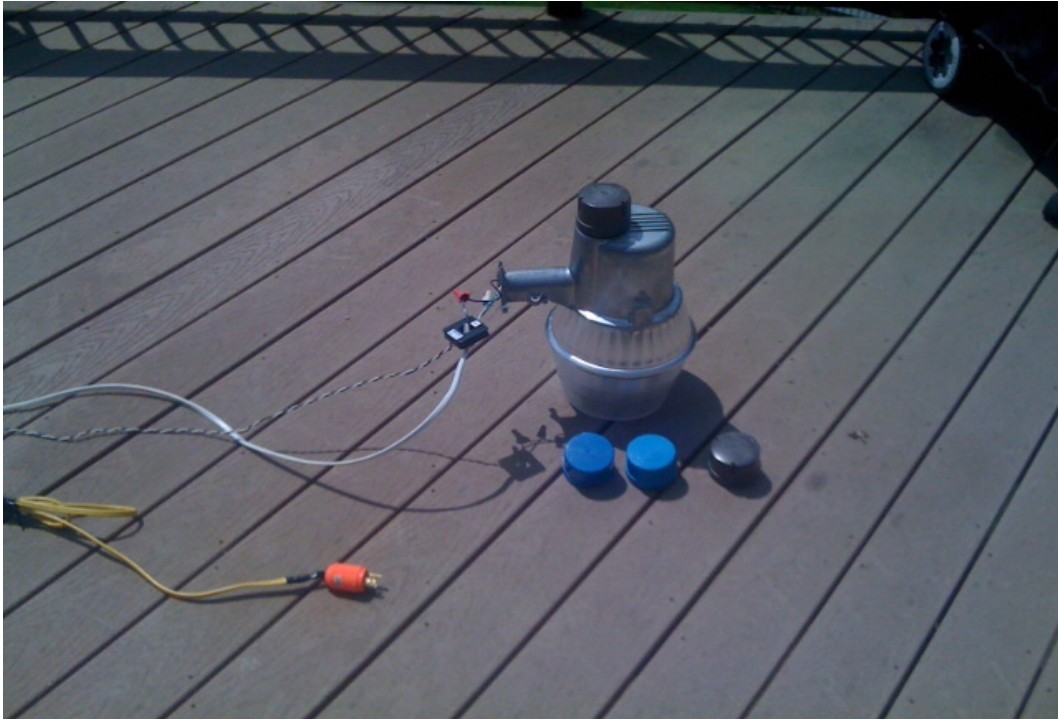
Figure 3-1 Utilitech70 Watt HPS Light (Also shown are the four photocells donated by the City of Rocky Mount and the City of Concord in blue and black)
