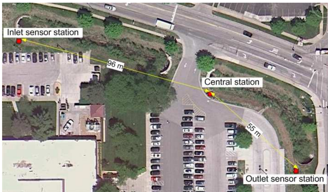
Figure 4.23 Map of the wireless network deployed in Mission, Kansas (Map from Google Imagery, Digital Globe, Sanborn, Map Data)
