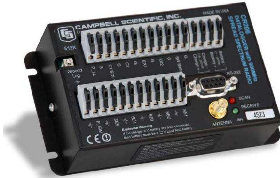
Figure 5.5 CR206 datalogger with spread spectrum radio from Campbell Scientific, Inc.
