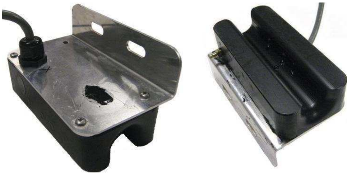
Figure 4.3 Prototype of the 4 th generation optical sensor
