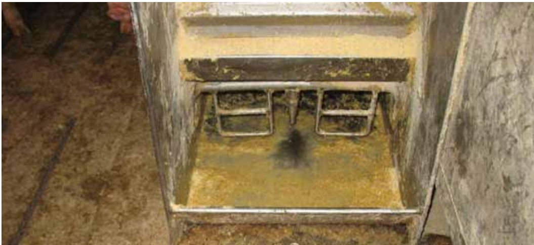
Figure 2. Wet-dry feeder at setting 10 with a 0.75-in. opening and \approx 57\% pan coverage.
