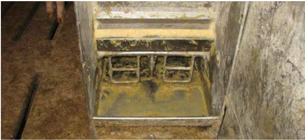
Figure 1. Wet-dry feeder at setting 6 with a 0.50-in. opening and \approx 35\% pan coverage.
