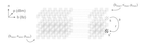
FIGURE 6.1: Three-dimensional state-space used to model the joint power and rate allocation problem as an MDP. Axes represent each constituent element of the available states of the MDP: beaconing rate, estimated number of neighbors, and transmission power.
