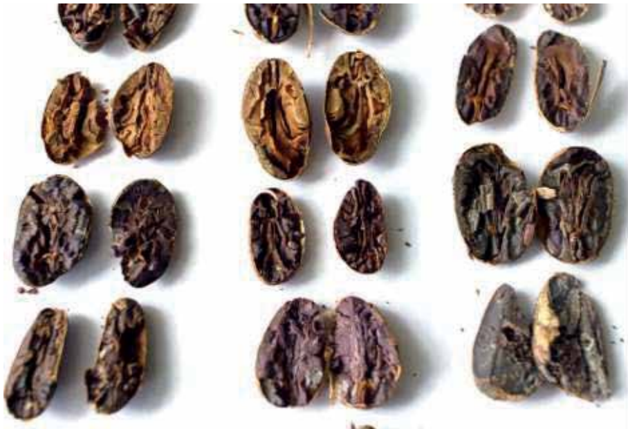
Figure 1. Cutting test of cocoa beans from various cocoa-producing areas of Venezuela, representing fermented, slightly fermented, unfermented, and damaged beans.
