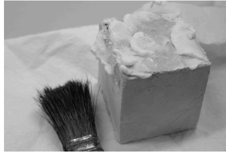
Fig. 4- Cubic limestone specimen with edge 5 cm treated with nano-gel
