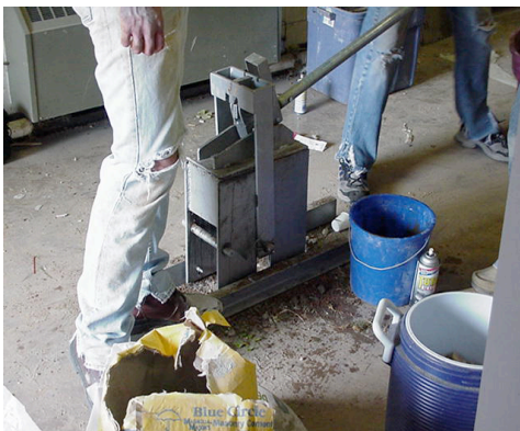
FIG. 3 Four steps in the process of creating compacted soil stabilized brick using a Cinva Ram. Architecture students at the University of Kansas under the direction of Professor Nils Gore. Photo by permission of Professor Gore.
