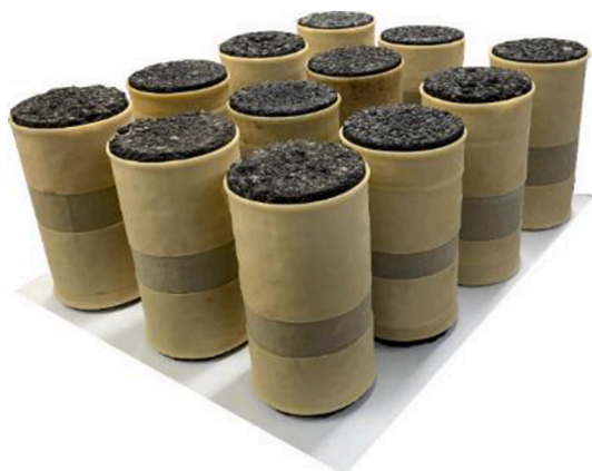
Fig. 2. Detail of the specimens curing under partially sealed conditions.
