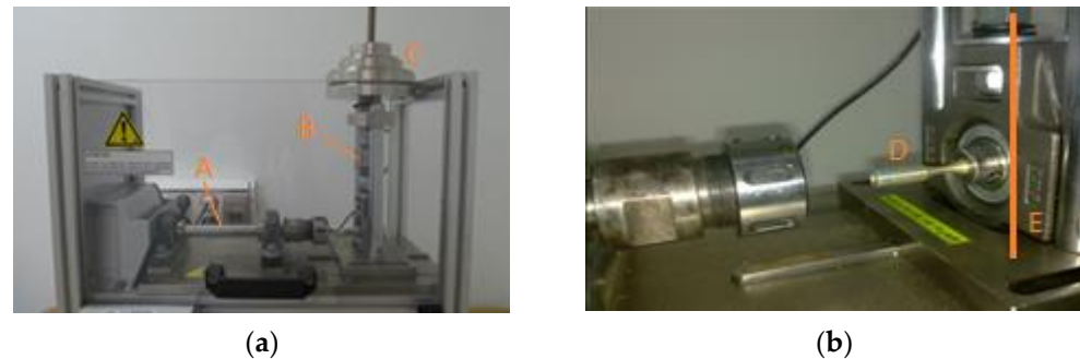
Figure 1. Device used for the test (a) A more detailed view of the same device (b). In the figure, A is axis of rotation linked to the motor at the far left of the figure, B the force transducer, C the masses, D the sample and E the load axis at the end of the specimen.
