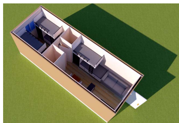
Figure 5.- Type-2 housing unit
