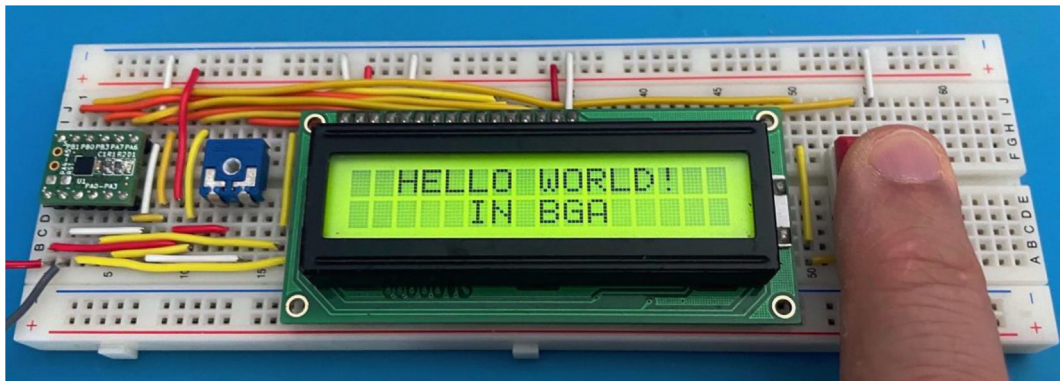
Fig. 13. UFBGA \mu -breakout board functional test.
