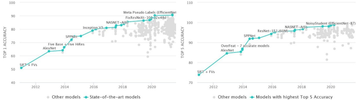
Figure 5 – Evolution of Image Classification models on ImageNet dataset: Top 1 Accuracy (left) and Top 5 Accuracy (right) (Facebook AI Research, 2021)
