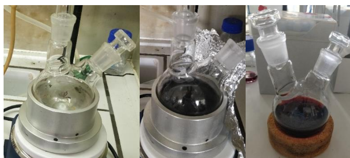
Figure 4.1 – Illustrative image of the colour change that occurs upon the addition of Au chloride.
