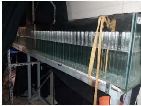
Figure 3.2: (a) Plan view representation of tests configuration (b) view of the array of cylinders.
