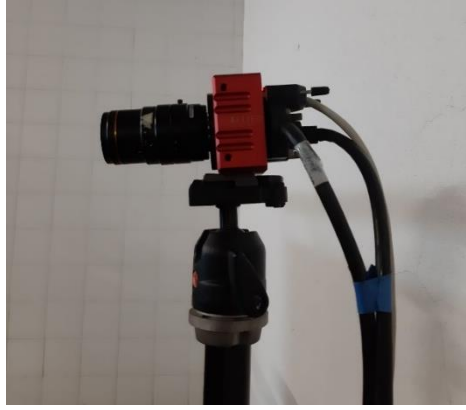
Figure 3.15: High speed camera Allied Bonito CL-400B/C.
