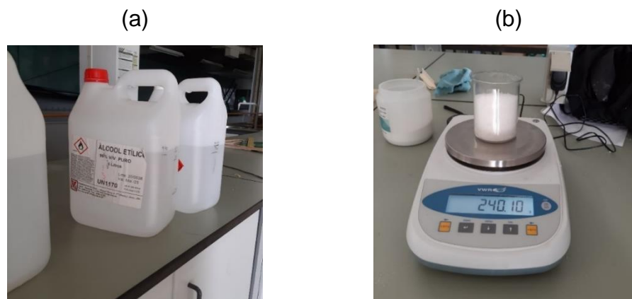
Figure 3.6: Measurements: (a) alcohol measurement with bidon; (b) salt measurement with digital scale.
