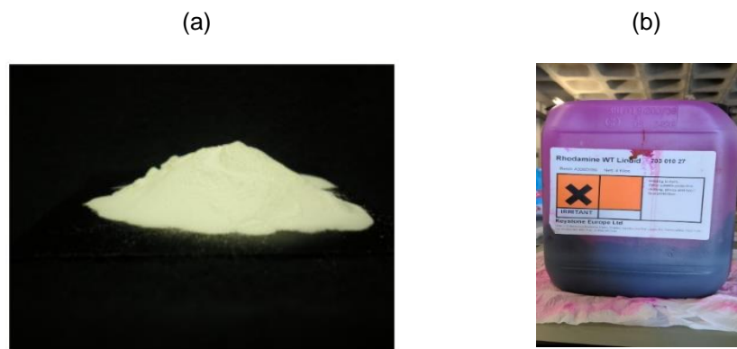
Figure 3.8: (a) Polyamide Seeding Particles; (b) Bidon full of rhodamine.
