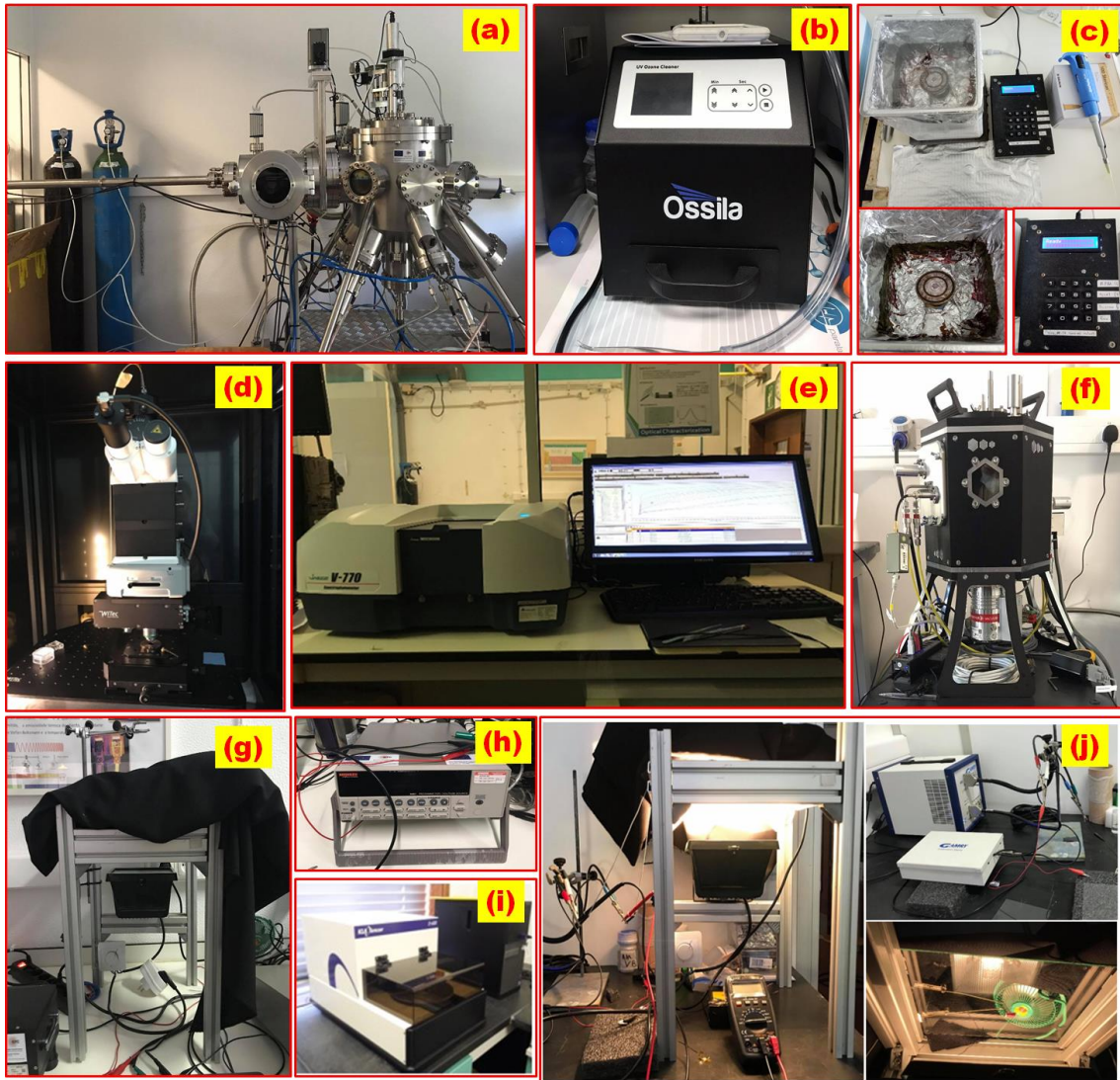
Figure A7 | Images of the instruments used in this research work (a) RF Sputtering from MANTIS system (b) UV-ozone cleaner from Ossila (c) Digital spin coater from Ni-Lo Scientific (d) Atomic Force Microscopy step up (ALPHA RAS 300) from WTec (e) UV-VIS-NIR Spectrophotometer JASCO V-770 (f) Thermal Evaporator System from (g) Self-designed solar simulator with halogen Lamp (h) Voltage source meter from Keithley (i) Surface stylus profilometer (ALPHA D-600 Stylus) from KLA Tencor (j) Impedance measurement setup include a light source (Reference 3000™ potentiostat/galvanostat from Gamry)
