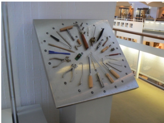
Figures 6 and 7 — Staatliches Institut Fur Musikforschung in Berlin. Educational exhibits showing the tools used in piano construction and the interior structure of a modern piano. Photo by Alcina Cortez, March 6, 2014.
